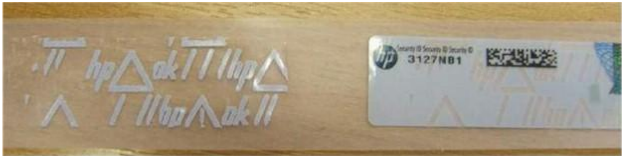
Figure 8: Adhesive left behind on product (left) and signs of tampering on label (right)
